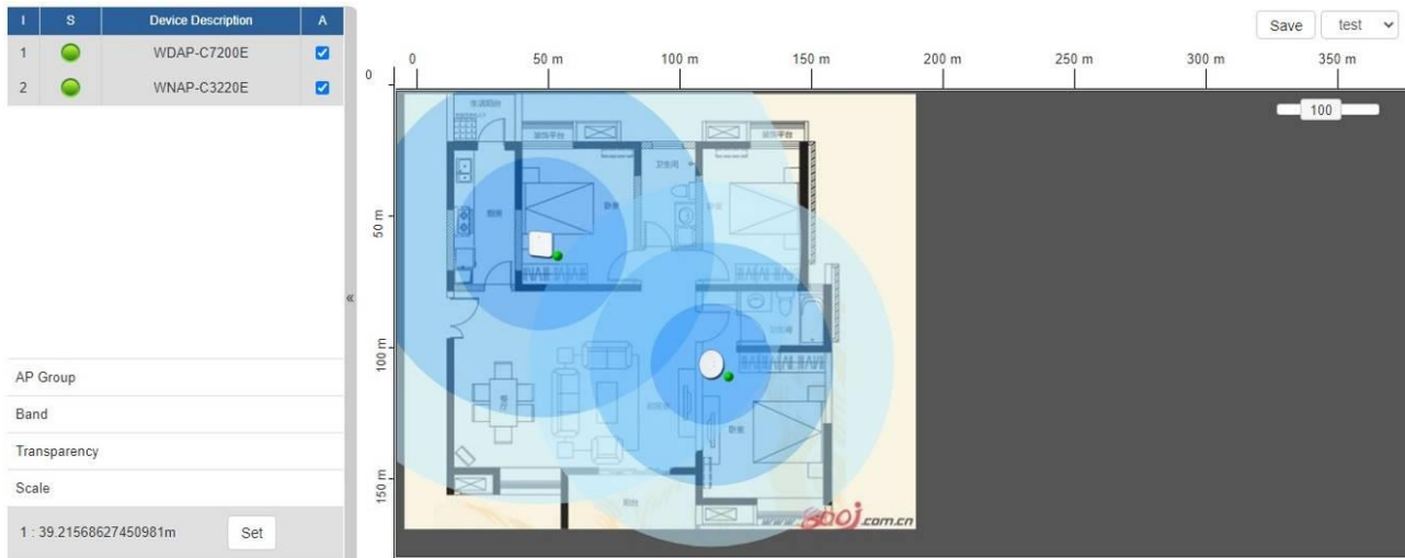
Figure 4.8-15 the simulator page of the wireless signal strong of AP
